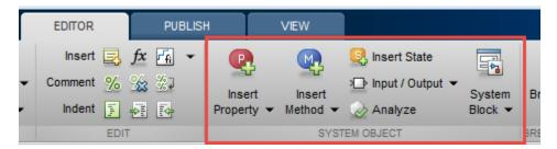
These coding tools are available when you open an existing System object or create a new System object with **New > System object**.
